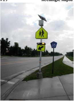
The RRFB is a rectangular shaped, high intensity signal head, which flashes in a wig-wag, rapid flickering pattern. The alternating signals provide direct, ultra-bright concentration as well as wide-angle intensity. The beacons are pedestrian activated: push button or passive detection
